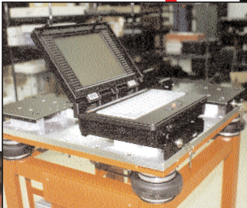
• SCR-350 on Test Table testing computer parts
