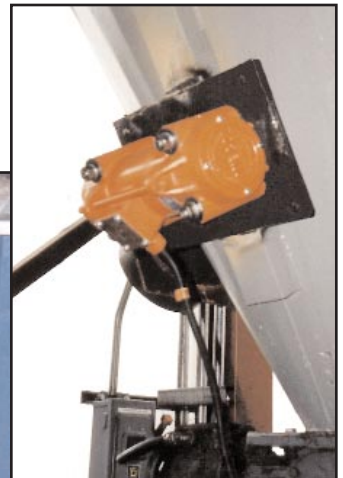
• SCR-400 on Stainless Steel Hopper
